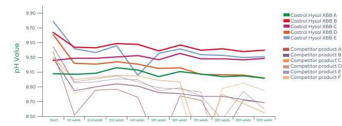
Castrol in-house microbiological test method. Occupation with bacteria and fungi isolated from field used oil samples.
