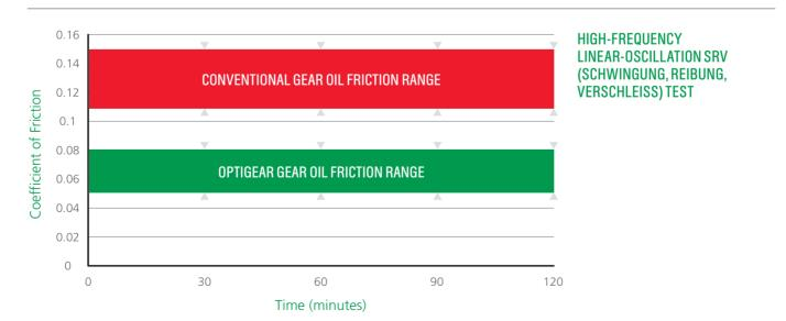
SRV test results show coefficients of friction of about 0.05 to 0.08 with Castrol Optigear compared to about 0.11 to 0.15 for conventional gear oil.
