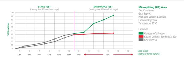
On pre-damaged gears (shown up to stage 10 on the left of the graph), further micropitting and gear damage can be minimised by switching to Castrol Optigear. However, with conventional gear oils, the damage continues to propagate and would lead to eventual failure.
