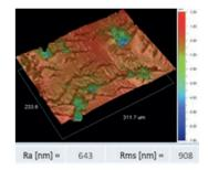
\* Independent MPR testing carried out by Powertrib showed weight loss was less than half that recorded with the use of a well-known conventional non-PD oil from a competitor.
